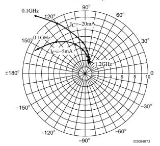
$\begin{array}{l} S22e: V_{\mbox{\scriptsize CE}} \!\!=\!\! -10V \\ f \!\!=\!\! 100\mbox{\scriptsize MHz}, 200 \mbox{\ to\ } 1200\mbox{\scriptsize MHz} (200\mbox{\scriptsize MHz\ step}) \end{array}$
